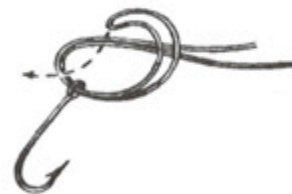
2. Let hook hang loose and tie overhand knot in doubled line.
