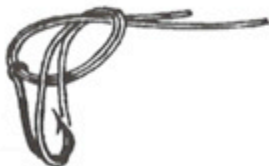
3. Pull loop of line far enough to pass over hook, swivel or lure.
