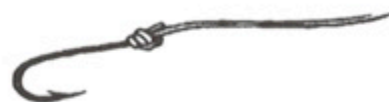
4. Pull tag end and standing line to tighten. Moisten before fully tightening. Clip tag end.
